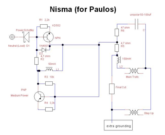
both coils wound on a little AM ferrite cores from radios
