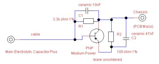
works with cables up to 0.8m long proposed transistor BD140 screwed to chassis
