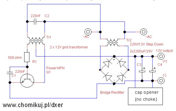
Self Sustaining Power Supply 12VDC/230VAC (solid state)
