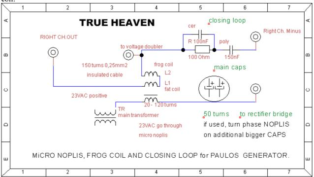
Most of amplifiers will work with 150nF cap and a resistor between 50-100ohm.
