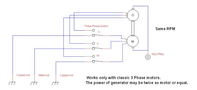
Self starting Qmogen proposition. You may use three groundings though they must be different (magnetism problem). With some modern motors all grounding may be connected to one and no matter of used material – any steel rod.
