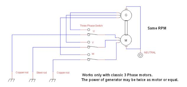
Self starting Qmogen proposition. You may use three groundings though they must be different (magnetism problem). With some modern motors all grounding may be connected to one and no matter of used material – any steel rod.
