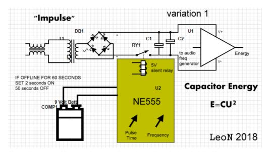
May be added to a ground line in symetric power supplies or other classic supplies, in i.e. Audio Amplifiers. Works only with a 0,1-1F overall supply.
