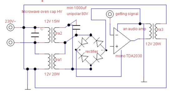
you may use other unipolar capacitor from a motor (the higher capacitance in uF). Tra3 is TS6/63. Normally use capacitor in power supply – the schematic lacks it. The unipolar cap used on ac line could have lower capacitance.
