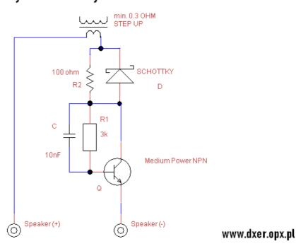
**STEP 4.** Trigger the transformer with the right noise. Set your volume to such level that you achieve the right voltage on your transformer output. This you will connect into AC IN of your device. Watch out the potentiometer! To get the right 50hz hum noise you may put a long wire into the left in or put the signal from phase via resistor divider like 500k a 1k and take the signal via poly cap like 1uF. This is better option. I was trying 1MOHM and 2.2k divider and it worked for me.
