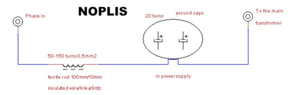
Wound up to 300 turns on ferrite core and caps. More does not count much for efficiency.
