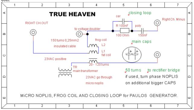
Most of amplifiers will work with 150nF cap and a resistor between 50-100ohm.
